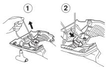
• Undo the screw in the centre of the pulley and remove the pulley. Insert and fasten a new starter cord to the pulley. Wind approx. 3 turns of the starter cord onto the pulley. Connect the pulley to the recoil spring so that the end of the spring engages in the pulley. Fit the screw in the center of the pulley. Insert the starter cord through the hole in the starter housing and the starter handle. Make a secure knot in the end of the starter cord.
